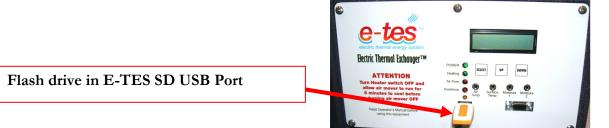
4. Press and hold both the UP button and DOWN button while your turn the power switch ON.
